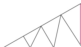
Figure 29: Mono-pitch truss - diagonal bracing to end vertical member
