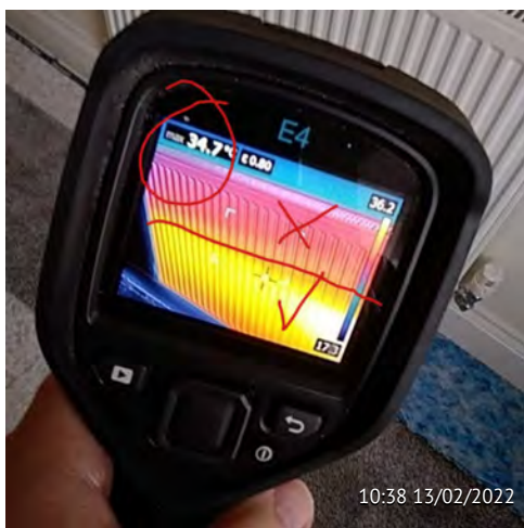
108 Landing trade Plumber Low radiator temp Radiator requires bleeding
