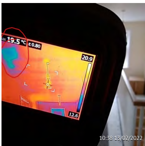
109 Landing trade Thermal Imaging Builder Builder to investigate and comment on results of thermal imaging .... Suggests insulation is not consistent at this point in loft
