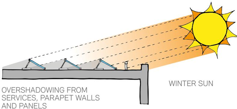
OVERSHADOWING FROM SERVICES, PARAPET WALLS AND PANELS
