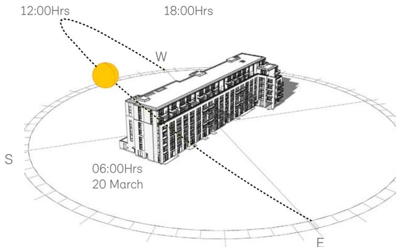
✅ ENVIRONMENTAL MODELLING OF SOLAR GAIN AND OVERHEATING
