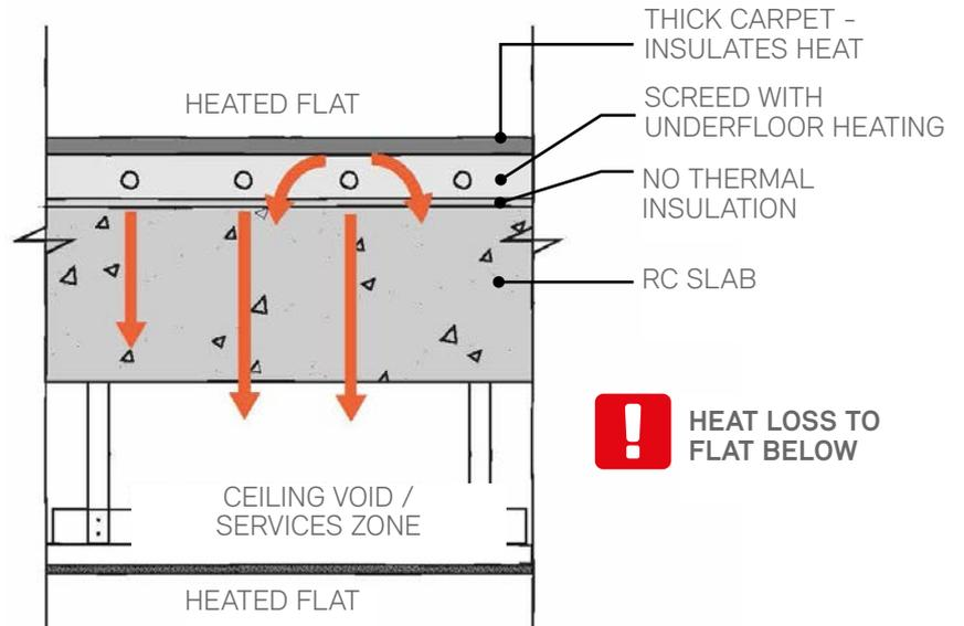
LACK OF INSULATION IN TYPICAL SEPARATING FLOOR BETWEEN FLATS
