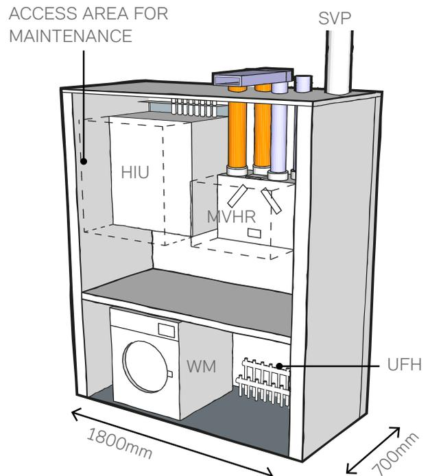
WELL DESIGNED HEATING/VENTILATION CUPBOARD IN AN APARTMENT
