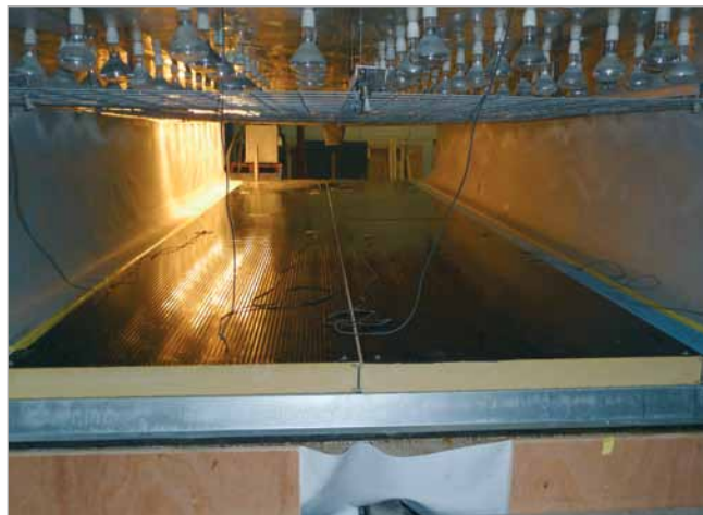
Commencement of heat cycle to upper surface of large sandwich panel
