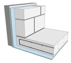
Tanked protection - External waterproofing with protection
