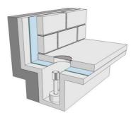
Drained cavity – water resistance reliant on collection and disposal of water through cavity drainage system
