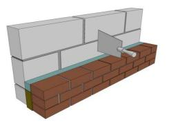
Clean cavities with the removal of all mortar droppings are particularly important in exposed areas and also where partial cavity fill is used. Additionally the width of the residual cavity should be not less than 50mm
