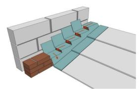
Where the roof abutments at an angle with the wall, preformed stepped cavity trays should be provided. DPC's below the coping should be supported above the cavity to prevent sagging. A specific dpc should be chosen in relation to each individual site and its needs in order to achieve a good key with the mortar.
