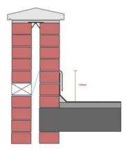
Cavity trays should be provided at abutments of cavity walls and roofs. This will guarantee that any water penetrating the cavity does not enter the enclosed area. This only applies where the roof is over an enclosed area, including attached garages, but does not apply to open car ports and or open porches.
